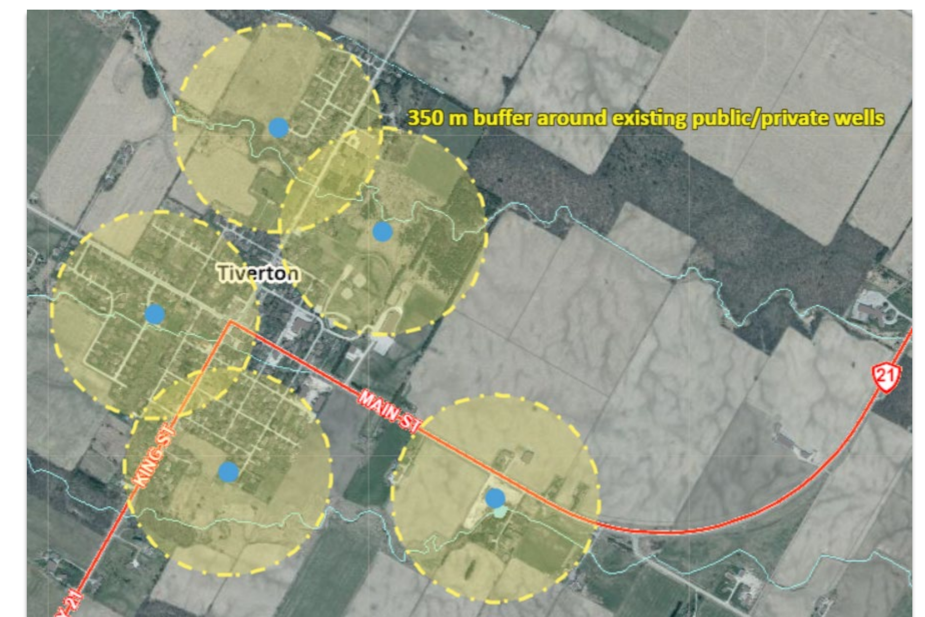
Minimum of 350 m setback required from existing wells in and around Tiverton to avoid interference. New wells will likely need to be located outside of the community.
